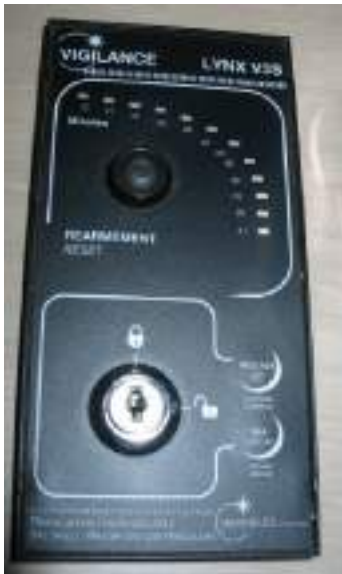
Figure 5-30 Bridge Navigational Watch Alarm
