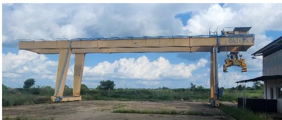
Gantry Crane with Lifting Clamp
